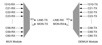
Note: The above figure is the wiring diagram of MT2010-DWDM-MUX40-CH21-CH60-MG-00.
